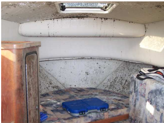
Photo 3: Mold and mildew in main cabin
